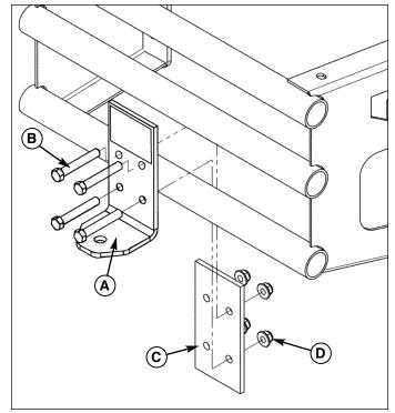
Figure 1. Install Hitch Kit
